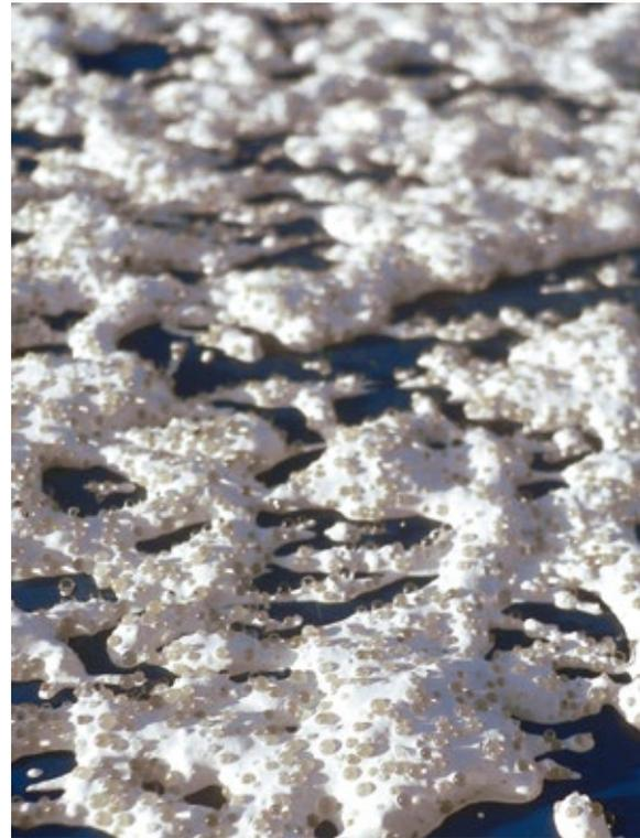
Reflective glass beads on top of a DEGAROUTE® based road marking
